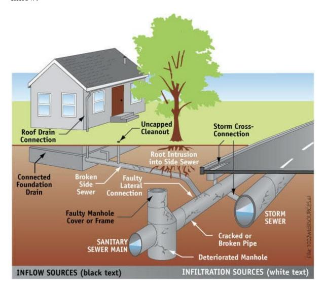
Inflow occurs when rainwater is misdirected into the sanitary sewer system instead of storm sewers. Examples are: roof leaders, yard and area drains, manhole covers, sump pumps, and cross connections from storm drains. The remedy for inflow is to remove improper connections to the sanitary sewer system.
