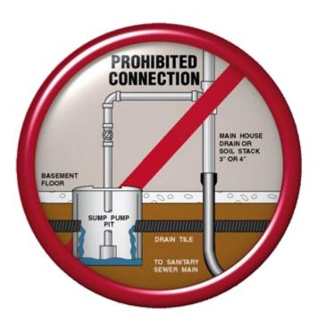
Shows a sump pump illegally connected to sanitary sewer. This is not allowed in Village of New Concord. The Village appreciates your help.
